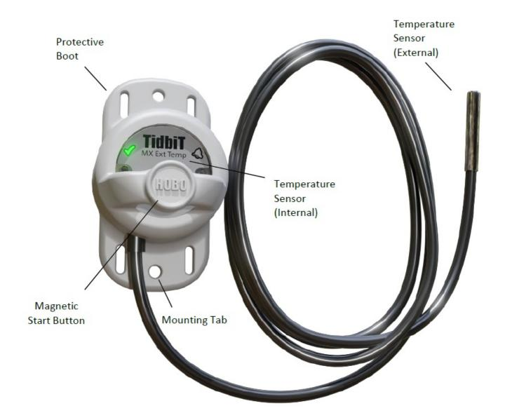
**Protective Boot:** This waterproof cover protects the logger during deployment. It has two mounting tabs and a built-in magnet to use with the logger's internal reed switch (see Deploying and Mounting the Logger).
