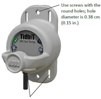
Use cable ties with the slots; slot dimensions are 0.28 cm (0.11 in.) wide x 0.86 cm (0.34 in.) long
