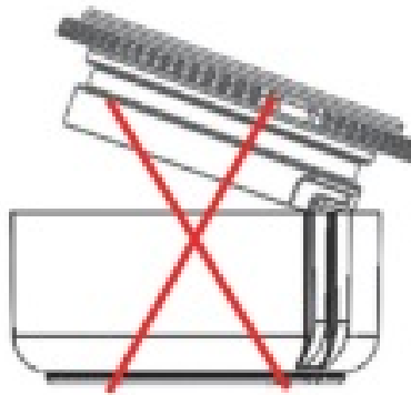
Battery Cover Side View, Incorrect Assembly
