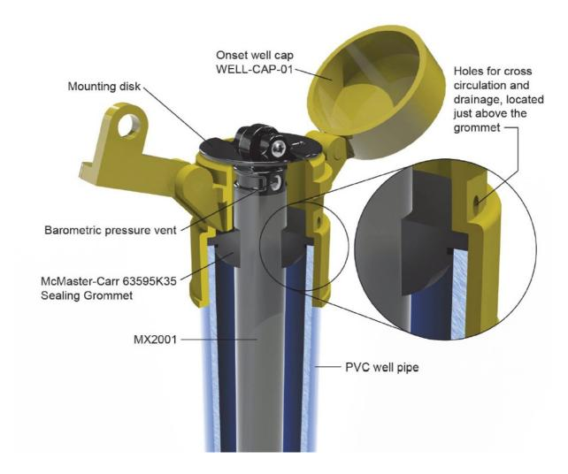
If your well must remain sealed or there is no way to avoid a continuous saturated environment, use non-vented water level loggers, such as the HOBO U20 or U20L water level loggers.
