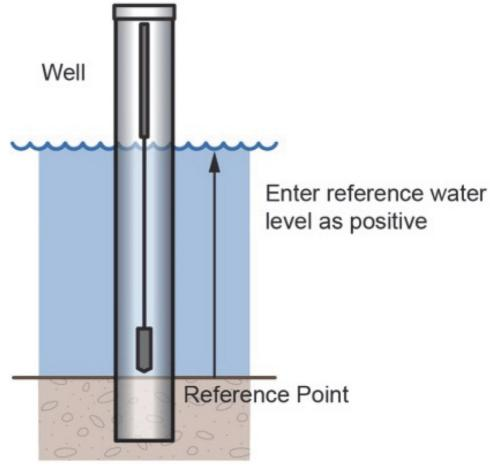
• If you are using the sensor as the reference point as shown below, enter the reference water level in the app as zero and start the logger before the sensor is in the water. The logged water level readings will represent the height above the sensor.
