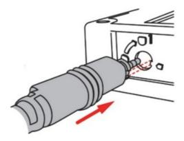
For other types of external analog sensors, insert the sensor plug into an analog sensor port.
