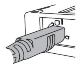
The flat part of the plug will be facing up when properly installed.
