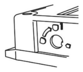
Using the diagram on the logger housing shown above as reference, insert the plug into the analog sensor port.
