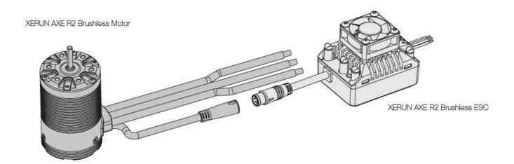
Please make sure that the two arrows align when connecting, otherwise you may damage the inner part of the connectors and cause the power system to function abnormally. Remember, never connect/disconnect them forcibly.
