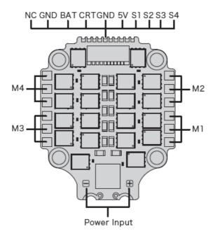
**Note:** Users only need to connect the throttle control wire and ground wire of the ESC to the corresponding ports (on peripheral devices like the receiver) when a single ESC needs to be programmed.
