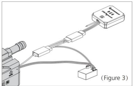
For the SEAKING 60A V4 ESC, due to its independent 3-pin programming interface, the method of connecting the program box or OTA programmer is different from other ESCs. The connection method is as follows.
