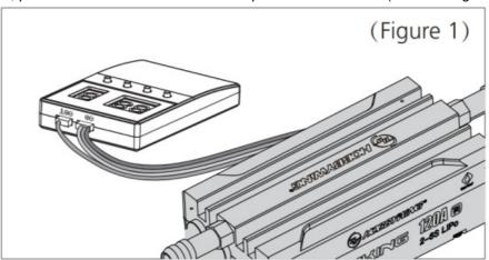
The OTA Bluetooth module is used to set the parameters:
