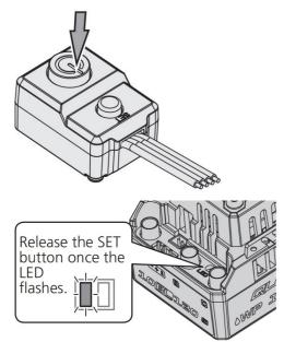
2. Start by turning on the transmitter with the ESC turned off but connected to a battery. Holding the "SET" button then press the "ON/OFF" button, the RED LED on the ESC starts to flash (The motor beeps at the same time), and then release the "SET" button immediately.
