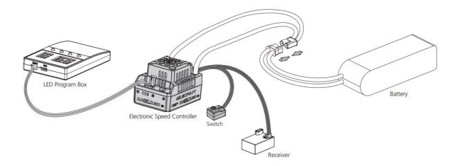
The program box needs to be connected to the independent programming port. Otherwise, it will not work!
