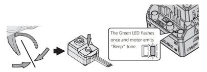
Move the throttle trigger to the end position of forward and press the SET button.
