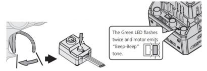
Move the throttle trigger to the end position of backward and press the SET button
