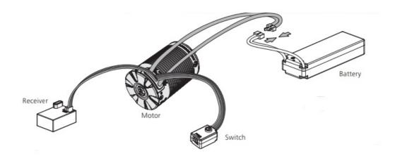
**Warning:** The power of the system is powerful. For the safety of you and other people around you, we strongly recommend that you remove the pinion gear before calibrating and setting the system, and turn on the control switch of the ESC when the wheel is suspended!
