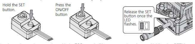
2. Start by turning on the transmitter with the ESC turned off but connected to a battery. Holding the "SET" button then press the "ON/OFF" button, the RED LED on the ESC starts to flash (The motor beeps at the same time), and then release the "SET" button immediately.
