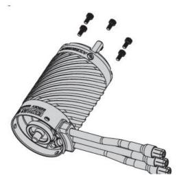
Mount screws for fastening the front end bell
