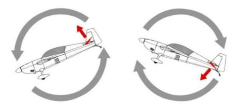
Check the gyro direction for Rudder Quickly move the nose of the airplane to the left around the yaw axis, the rudder surface should flap right as shown below.
