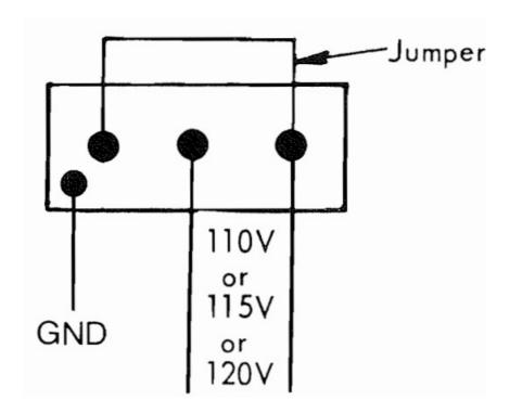
**CAUTION**: A three-pole toaster 120/208 V or 120/240V cannot be connected to a 2-pole 208V or 240V, 2-pole single phase system.
