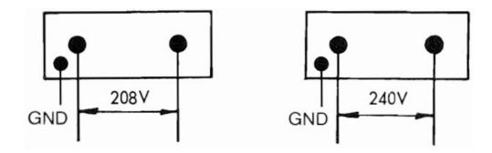
Two-wire single-phase power systems can be connected to the Model ET24 4-slice toaster as shown below. For such connections, a different model toaster (than the 3-pole model) is used – one that has a 2-pole, terminal board.
