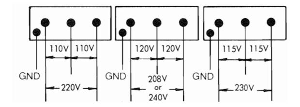
If 2-pole connections are to be used from these three pole systems, then a jumper must be used between the outside terminals in the toaster terminal box as shown: (The jumper is taped at the outside top of the terminal box should it be required).
