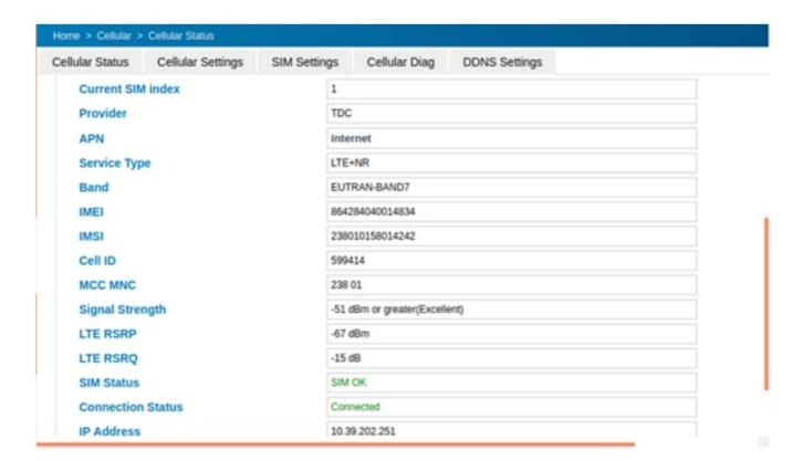
Please note the Cellular IP address allocated to the device.
