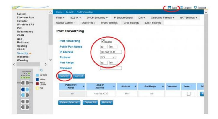
Please configure forwarding of port 80 TCP to LAN IP address 192.168.10.10 port 80. Press "Submit" and then "Save" to make the changes permanent.
