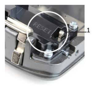
1. Reset-Hebel (reset-lever)
