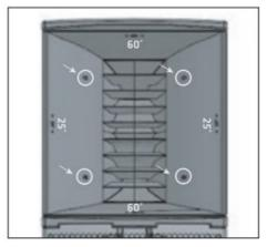
To get the best audio results when clustering LINEAR 9 210 LTAs, you will have to rotate the two adjacent horns to set them to a horizontal directivity of 25°. The angles are clearly marked on the horns.
