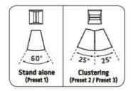
Select the appropriate preset on the back of the speakers for the given type of cluster.
