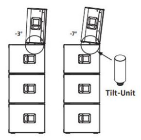
Heads up! When you stack speakers without using the Tilt Unit to fix them in place, be sure to secure the mid/high units – for example, with a lashing strap to hold them in place.
