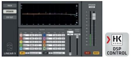
Screenshot of the remote DSP CONTROL software. You can download this software free of charge at the LINEAR 9 product page at <a href="https://www.hkaudio.com">www.hkaudio.com</a>. The speaker and DSP Out parameters are identical, but the powerful onboard DSP lets you configure each set independently.
