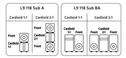
Both setups attenuate the rearward sound pressure level by up to 34 dB, and boost the forward SPL around 2 dB.
