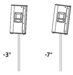
All Mid/High units are equipped with the HK Audio DuoTilt 3°/7°, a special type of pole mount for 35-mm speaker stands and poles that provides tilt angles of -3° and -7°.
