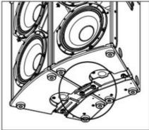
You can also fly one LINEAR 9 210 LTA or a cluster of two with the optional TB-210NQ tilt bracket. If you want to fly two speakers with this tilt bracket, you have to additionally secure the cluster with the bottom cluster couplers. This is mandatory:
