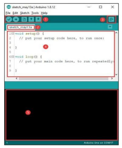
4. Tool bar contains some shortcut keys for the commonly used functions, asthe following table:
