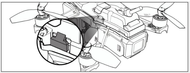
3. Once activated, the aircraft stays in bind mode for 20 seconds, then will returns to standby state after 20 seconds or a successful bind. Repeat the steps above if needed.
