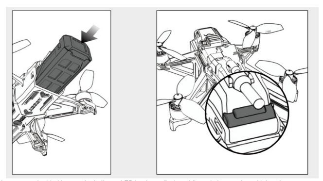
Long press the bind button, the indicator LED begins to flash rapidly and alternate in multiple colors.
