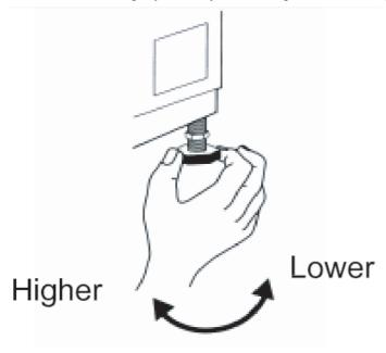
7. **Important:** tighten the locknut by turning it anti-clockwise towards the appliance casing.
