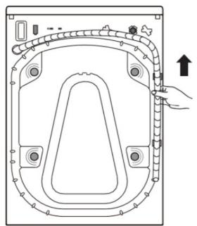
12. Connect the drain hose to the siphon or hook it over the edge of a sink by means of the "U" bend. Fit the "U" bend E, if not already installed, at the end of the drain hose.
