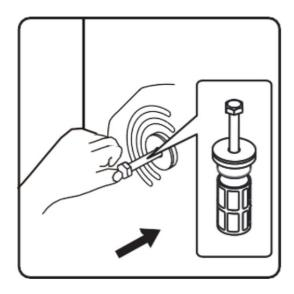
4. To ensure safety and reduce noise, you should install the transportation bolt cover supplied with the unit (see the annex accompanying the unit). Lean and place the transportation bolt into hole and press it following the shown direction until it clicks.
