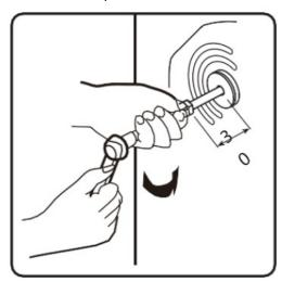
3. Pull out transportation bolt together with rubber part and plastic part
