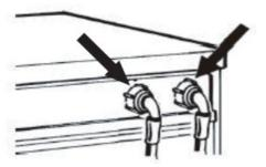
9. Screw by hand the inlet hose onto the tap, tightening the nut.
