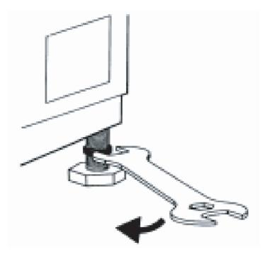
6. Lift the machine slightly and adjust the height of the foot by revolving it.
