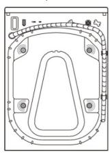
2. Push two transportation bolts on horizontal direction inward and loose transportation bolt.
