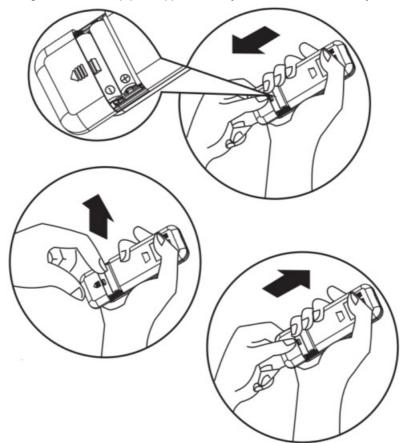
Reattach the cover by sliding it back into position.
