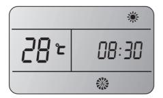
You can adjust the real time by pressing CLOCK button, then using  $\triangle$  and  $\triangledown$  buttons to get the correct time, press CLOCK button again the real time is set.
