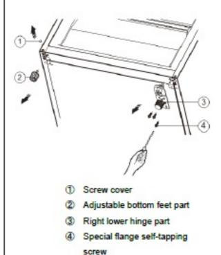
Replace part ③ to the left side and fixing it with the screws ④ . Replace part ① and part ② to another side and fixing it.
