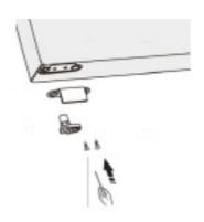
Lay the freezer on soft foam packaging or similar material. Remove part ① part
