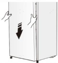
Replace the lid by fitting the upper hinge core into the upper door's hole, securing it with the 3 screws.
