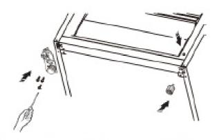
Note: 1. You need move hinge axis from hole ① to ② , move adjustable bottom feet part from hole ③ to ④ before transfer.
