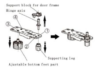
Set the door into its new place making sure the pin enters the bushing at the lower frame section.
