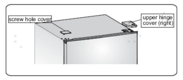
2. Remove the three screws as follow diagram. Lift the right upper hinge part.
