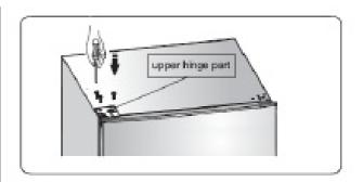
Put the screw hole cover and upper hinge cover ( left ) as follow diagram.
