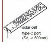
You can charge the remote by exposing the solar cell to light or using a USB type-C cable(not provided).
