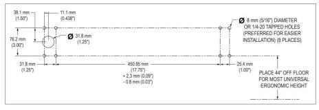
2. Install the left hand wall bracket first using four of the provided 1/4-20 screws, washers, and nuts as shown. Tighten all screws until the gasket is compressed to 1/16" to 3/32" thick.
