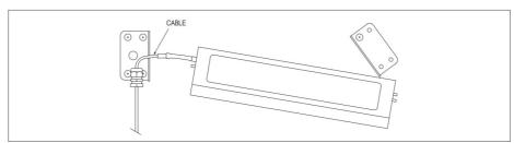
5. Swing the right hand wall bracket into place, trapping the keyboard as shown.
