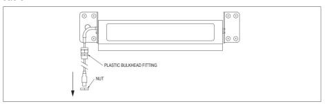
8. Insert the cable and fitting through the hole in the left hand wall bracket. Tightly reinstall the nut from the rear. Push the cable through as far as it will go, then tighten the cable gland nut from the front.
