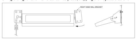
6. Finish installing the right hand wall bracket using the remaining three 1/4-20 screws, washers, and nuts. Tighten all screws until the gasket is compressed to 1/16" to 3/32" thick.
