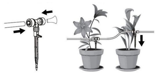
Turn clockwise to increase the flow rate; Turn counter- clockwise to reduce flow rate.
