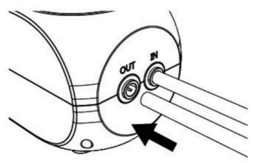
**Step5.** Connect the check valve to the water outlet near the pump. (Please install correctly in accordance with the flow direction.)
