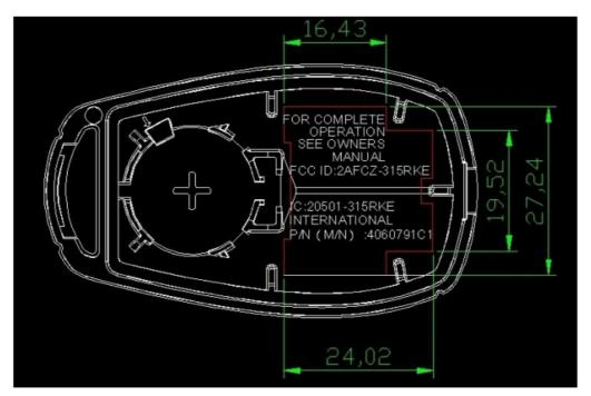
FCC ID is on the inner surface of shell
