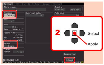
A 50 Hz measurement frequency is equivalent to 20 ms per cycle. When using the 5 ms/div time axis range and selecting to record 15 divisions, a 75 ms waveform can be monitored. (5 ms/div x 15div = 75 ms) This is equivalent to approximately 3.5 cycles.
