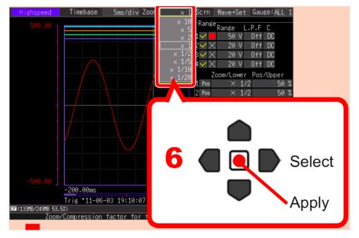
When the zoom ratio of the time axis is changed, the waveform printout will also zoom in or out accordingly.
