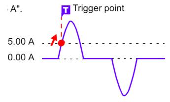
5. Press the START key to begin measuring. "Waiting for trigger" will be displayed until the set trigger conditions are met. When the trigger is activated, measurement will occur once.
