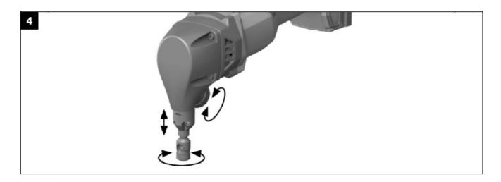
If necessary, the cutting direction can be turned right or left in steps of 45°.
