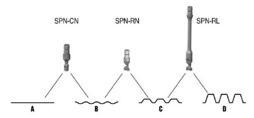
See the illustration for the correct combination of accessory tool and material to be worked.
