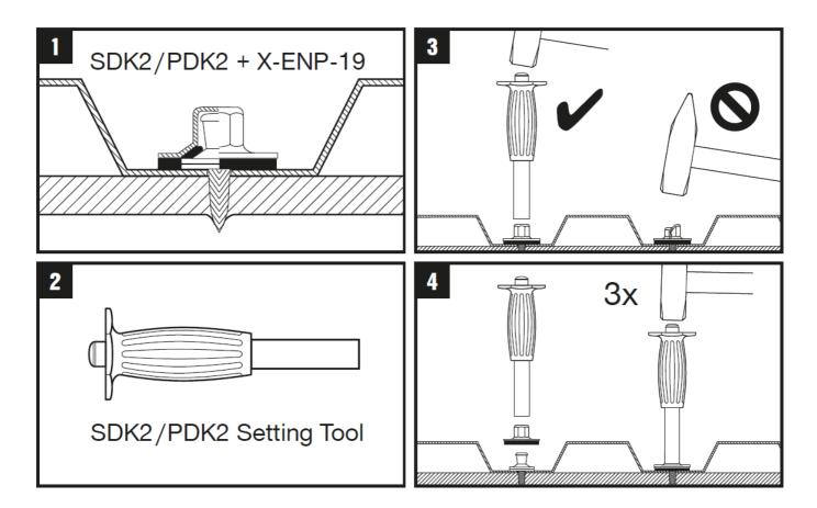
Sealing cap for nails used in exposed roofs and cladding
