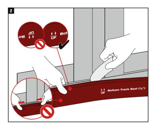
**Step 3**Ensure the seal is pressed tightly into the corner to prevent gaps.
