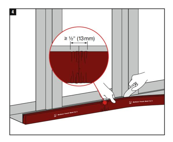
Step 5 For corner installations, ensure the seal is continuous and overlaps by at least 1/2'' (13mm).
