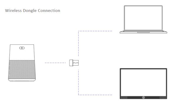
The default wireless receiver name is Multi-mic Speakerphone for wireless dongle connection.
