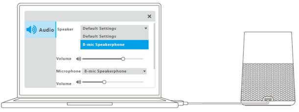
Plug the microphone in the computer and run the conference/video software to use the device.
