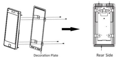
3. If you have to install the device outdoors, you should install a protec ve shield(op onal) for the device.
