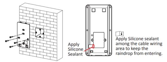
Align the device with the mounting plate and hang the terminal on the mounting plate.
