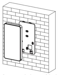
4. Use the supplied hex key to secure the 2 screws at the bottom of the device.
