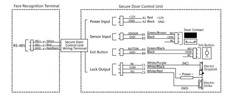
The secure door control unit should connect to an external power supply separately. The suggested external power supply is 12 V, 0.5 A.
