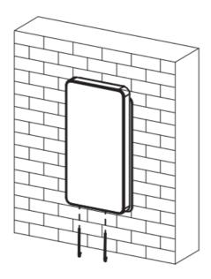
Apply Silicone sealant among the joints between the device rear panel and the wall (except the lower side) to keep the raindrop from entering.
