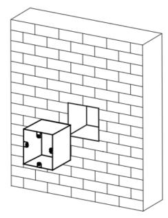
2. Use supplied screws to secure the mounting plate on the gang box.
