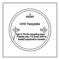
2. Fix the mounting base to the installation position according to the holes on the mounting template.
