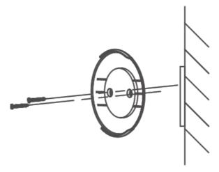
3. Line up and wedge the lower edge of the camera base with the mounting base and then push the camera to the mounting base to secure it.
