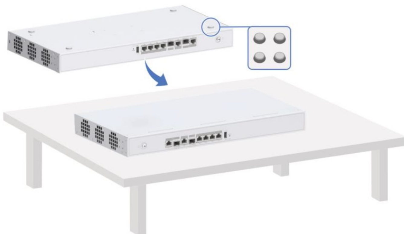
Figure 1-1 Mount Device on Workbench
