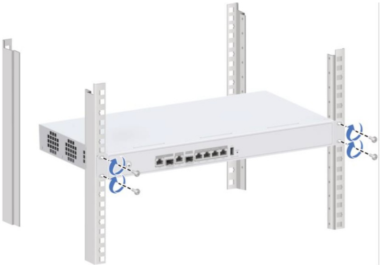
Figure 1-4 Install Device in Rack
