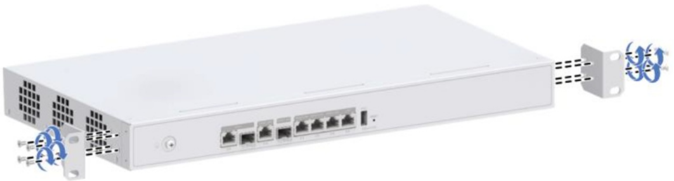
Figure 1-3 Attach Mounting Brackets
