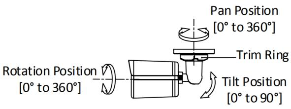
Figure 2-10 3-Axis Adjustment
