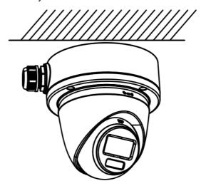
Figure 2-21 Combine Junction Box Cover with Body
