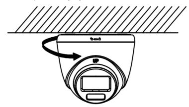
Figure 2-14 Snap Camera into Gang Box
