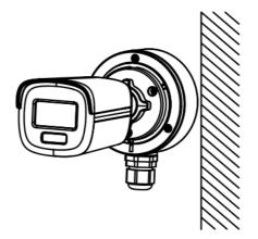
Figure 2-7 Fix Junction Box Cover on Its Body
