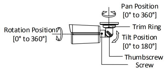
Figure 2-3 3-Axis Adjustment
