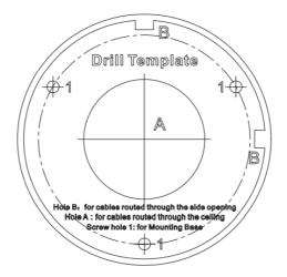
Figure 2-4 Drill Template for Junction Box
