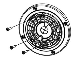
Figure 2-17 Install Gang Box to Junction Box Cover
