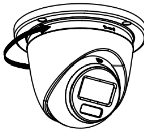
Figure 2-46 Snap the Camera into the Gang Box
