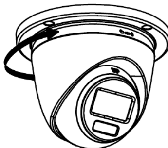
Figure 2-46 Snap the Camera into the Gang Box
