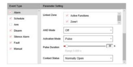
Note: AND Mode means only all zone triggered, then relay will output
