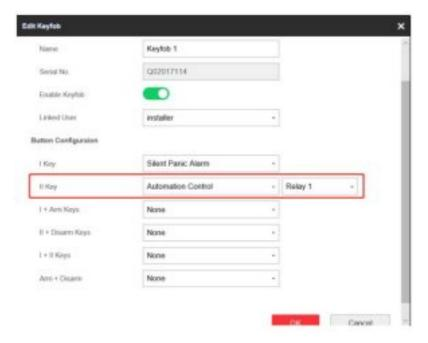
3. Configure Automation Control Device Event Type—Manual, select Activation Mode and Pulse Duration.
