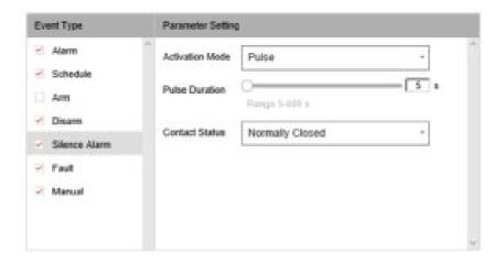
Fault: System Fault Event will link the Automation Device open or close
