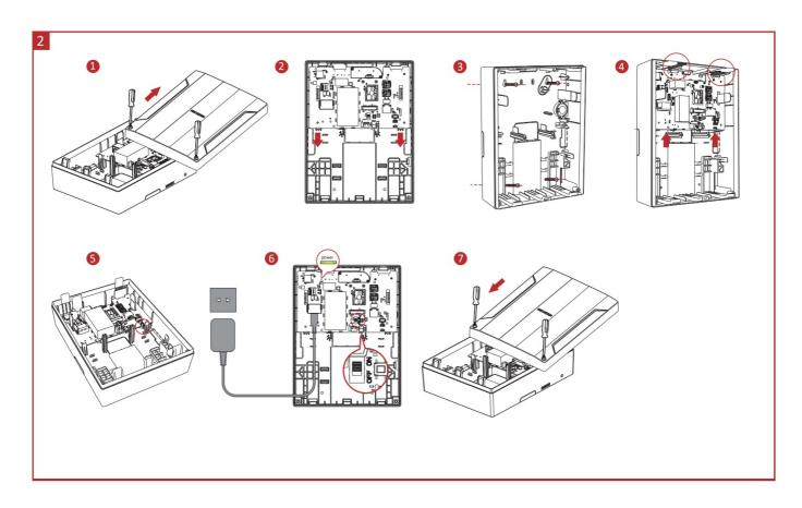
Note: Power down the control panel before installation.
