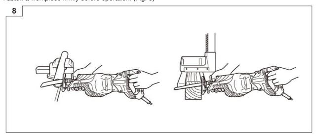
• When cutting metallic materials, use proper machine oil (turbine oil, etc.). When not using liquid machine oil, apply grease over the workpiece.
