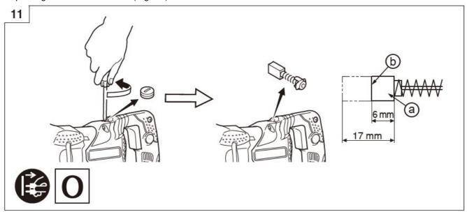
The motor employs carbon brushes which are consumable parts. Since an excessively worn carbon brush can result in motor trouble, replace the carbon brushes with new ones having the same carbon brush No. shown in the figure when it becomes worn to or near the "wear limit". In addition, always keep carbon brushes clean and ensue that they slide freely within the brush holders.
