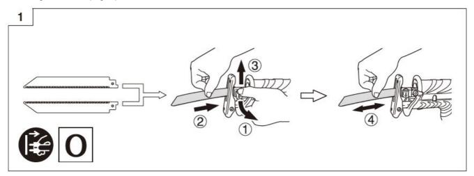
This unit employs a detachable mechanism that enables mounting and removal of saw blades without the use of a wrench or other tools.
