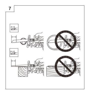
If you cut a large pipe, large block of wood, etc., that exceeds the cutting capacity of a blade; there is a risk that the blade may contact with the inner wall of the pipe, wood, etc., resulting in damage.
