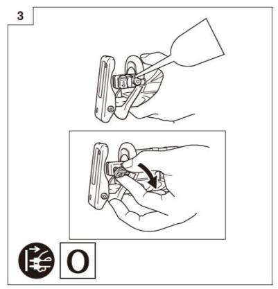
Continued use of the tool without cleaning and lubricating the area where the saw blade is installed can result in some slack movement of the lever due to accumulated sawdust and chips. Under the circumstances, pull a rubber cap provided on the lever in the direction of an arrow mark as shown in Fig. 3 and remove the rubber cap from the lever. Then, clean up the inside of the blade holder with air and the like and carry out sufficient lubrication.
