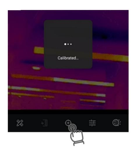
**Note:** You can calibrate device manually, and your device also periodically performs a self-calibration to optimize image quality and measurement accuracy. In this process, the image will pause briefly and you'll hear a "click" as a shutter moves in front of the detector. The self-calibration will be more frequent during start up or in very cold or hot environments. This is a normal part of operation to ensure optimum performance for your device.
