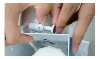
3. Open the tap water to wash the 1st and 2nd stage filters for around 2 mins till the outlet water is clear enough; Meanwhile, put a bucket under 3rd stage housing in case. The 2nd GAC filter head, contacting the white round rubber pad, shall be put upward
