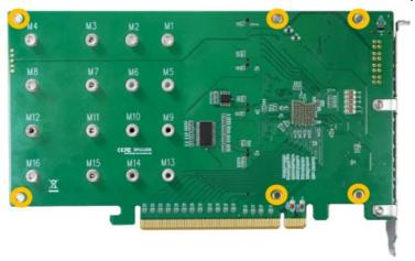
**Note** Make sure the aluminum cover is properly aligned with the controller board (PCB), and that it makes full contact with the thermal pad, before refastening it to the SSD7204. If the cover is improperly installed, the fan and thermal pad will be unable to suficientlycooltheNVMe SSDs and controller componentry, which may result in damage to the SSDs or controller hardware, performance loss, unstable, and the loss of data.
