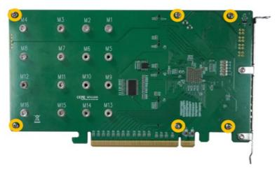
After removing the screws, carefully remove the heat sink from the SSD7104F.
