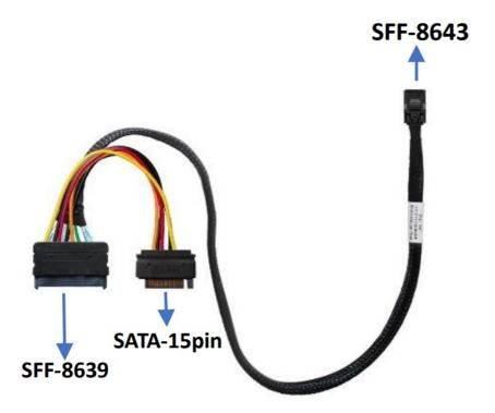
**Step 4:** Shown above is an SFF-8643 to U.2 SFF-8639 cable with a 15- pin SATA power connector. Connect the R1120 to the NVMe SSD's using the appropriate SFF-8643 cables. The SFF-8639 port should be connected to the NVMe SSD's U.2 port. The 15 pin SATA power connector should be connected the system's power supply.
