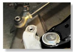
Remove the cotter pin, then remove the bolt and disconnect the tie rod end from the knuckle. (15mm) KEEP ALL FACTORY HARDWARE.
