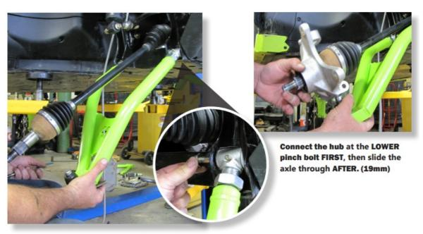
Connect the new lower arm at the frame using the factory hardware. NOTE: MAKE SURE THE BRAKE LINES ARE OUT OF THE WAY.
