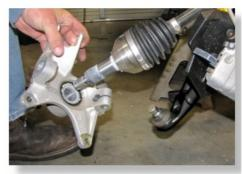
Remove the Lower Arm FIRST by removing the bolts at the knuckle (15mm) and the frame. KEEP ALL FACTORY HARDWARE.
