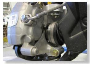
Secure the caliper to the knuckle by fastening the stock caliper mounting bolts. ENSURE THERE IS NO PINCHING OR BINDING OF THE BRAKE LINES.
