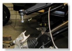
Disconnect the Upper arm by removing the cotter pin, then the bolts at the knuckle (19mm), sway bar, shock, and the frame. KEEP ALL FACTORY HARDWARE.
