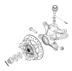
Remove the cotter pin, axle nut, and washers from the hub assembly, then remove the hub. (30mm)
