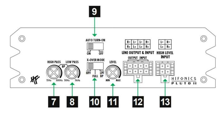
**7** HIGH PASS This controller limits the frequency downwards. Low frequencies that can damage a loudspeaker are cut off. The crossover frequency is adjustable from 15 Hz to 500 Hz.
