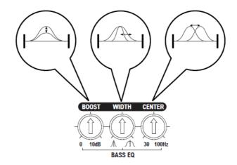
• Frequency: This setting is used for selecting the frequency you want to focus your enhancement on. The suggested enhancement is from 35-45Hz, but you should be careful not to set enhancement below the F3 or -3dB point of your sub/enclosure combo.
