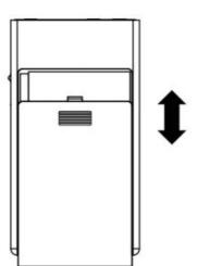
Open the back cover to change the amplifier card. In order to customize for different headphones, earphones and customers, HIFIMAN provides a variety of amp cards to choose from. Please see the following diagram for the steps to replace the amplifier card:
