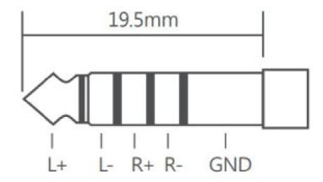
For 4.4mm Balanced to dual XLR connections, the balanced output should be as wired as follows:
