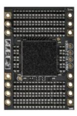
HYMALAYA is a discrete R2R DAC (digital-to-analog) module that is based on the FPGA algorithm. The combinations of its low audio frequency range, out-of-band noise, and low energy consumption make it a perfect match for high-performance audio equipment. The HIMALAYA DAC module supports the standard PCM music signal transmitted by the most common IIS (Integrated Interface of Sound) audio interface, with a maximum resolution of 24Bit.
