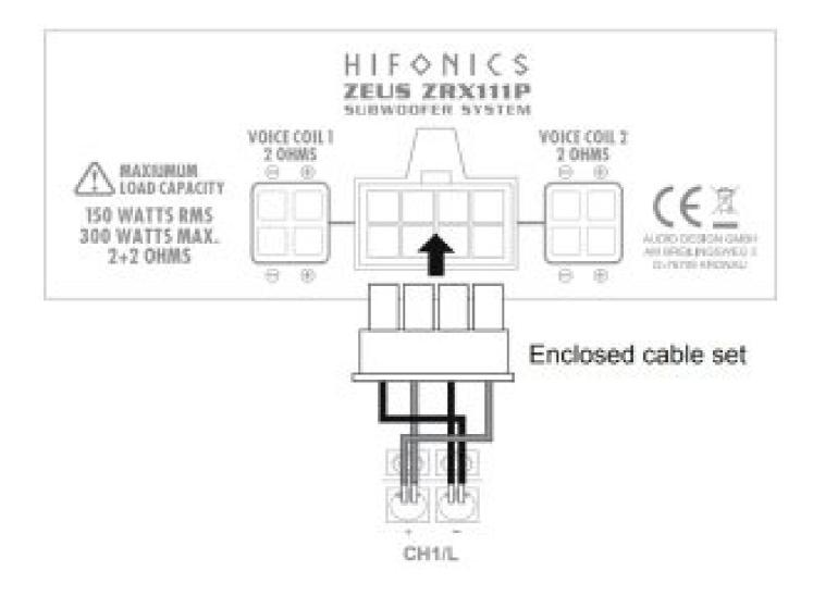
Connect the four cable ends accordingly to the loudspeaker outputs of the amplifier.
