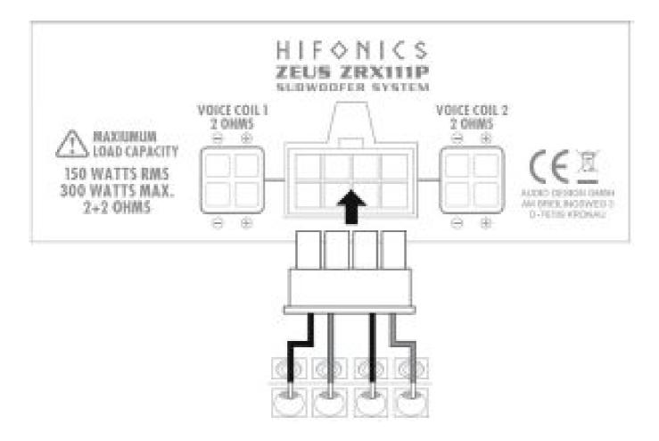
Connect the two cable ends of VOICE COIL 1 accordingly to the loudspeaker output CH1/L of the amplifie Connect the two cable ends of VOICE COIL 2 accordingly to the loudspeaker outputs CH2/R of the amplifier.
